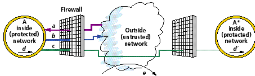
[Fig. 2] Domains A and A*, though parts of one organization’s network, are physically separate and communicate through an outside (untrusted) network. Firewalls can only control communication traffic to, from, or through that outside network--such as messages a, b, and c. They cannot control messages d and d’, which do not leave the protected networks’ boundaries, and connection e, which simply extends through the outside network.
